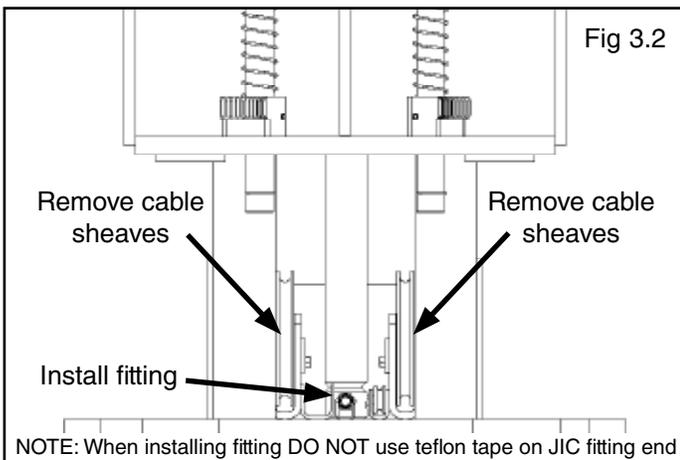
NOTE: When installing fitting DO NOT use teflon tape on JIC fitting end
