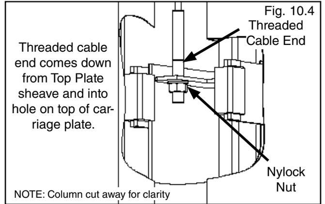
4. Insert the threaded end of the cable through the hole on top of the carriage. Place M18 washer and M18 Nylock nut on threaded cable end. Tighten cable nuts until taut, checking that both cables have equal tension. (See Fig 10.4)
