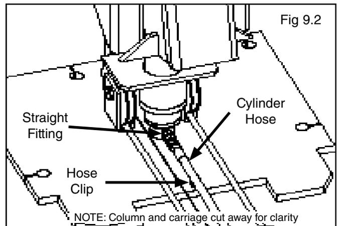
3. Route the power unit hose between the cylinder shaft and the equalizer sheave bracket. Route the hose through the hose clip. Failure to do so may cause damage or injury. (See Fig 9.3)
