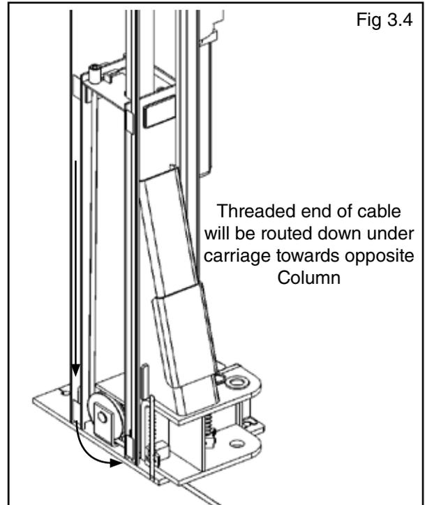
NOTE: Portions of Carriage and Column cut away for clarity
