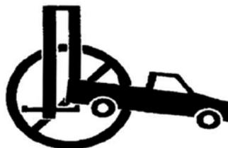
**NEVER LIFT ANY VEHICLE IN ANY MANNER WITH LESS THAN ALL FOUR (4) ARMS. RATED CAPACITY OF EACH LIFT ARM IS NO GREATER THAN ONE FOURTH (1/4) OF THE OVERALL LIFT CAPACITY.**
