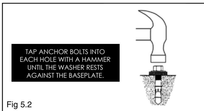
5. If shimming is required, insert the shims as necessary under the base plate so that when the anchor bolts are tightened, the posts will be plumb.
