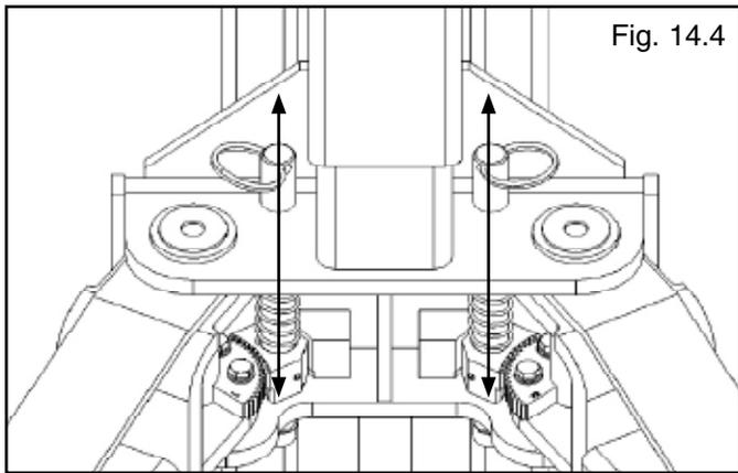
6. Ensure that the arms do not move when a force of approximately 100 pounds or less is applied laterally to the fully extended arms.
