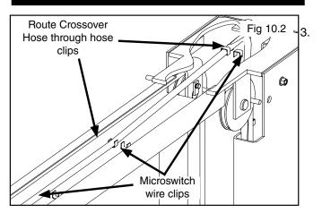
Route the Off Side cylinder hose (Crossover Hose) up through the post and across the Overhead Assembly, down the post and connect it to the bulkhead tee fitting. (See Fig 10.1 and Fig 10.2)
