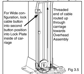
For Narrow configuration, lock cable button into Lock Plate inside of carriage
