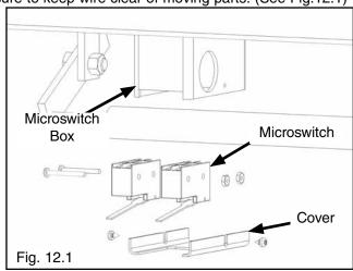
Note: Second Microswitch for 3 phase wired units ONLY. 3 phase Microswitch Kit can be found in the Power Unit shipping box.
