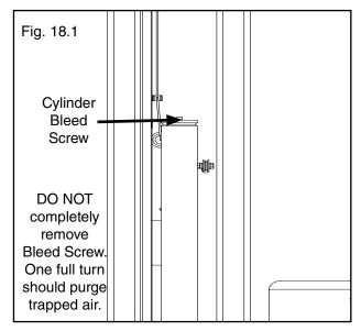
5. Lower the lift completely by pressing the SAFETY RELEASE handle inward then pressing the DOWN lever on power unit. Wait five minutes and repeat bleeding process one additional time.
