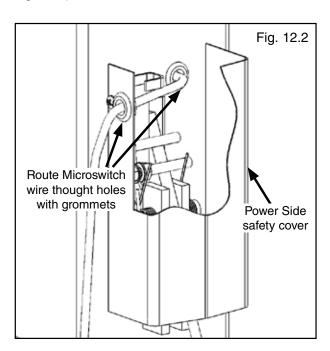
3. Route wire up through post and across Overhead Assembly through hole in Overhead Assembly into the Microswitch box. (See Fig. 12.3)
