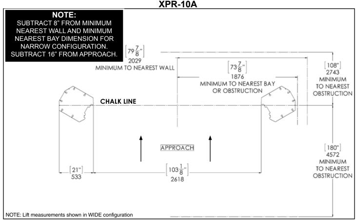
LIFT HEIGHT CLEARANCE NOTE: There must be a 1" MIN distance from top of lift to nearest obstruction.
