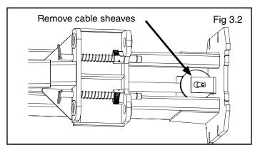
3. Identify the correct cable button on the end of each equalizer cable that corresponds to your desired lift configuration. Route the button around the bottom sheave and secure at the carriage lock plate located inside each carriage.
