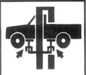
Use height extenders when necessary to ensure good contact.
