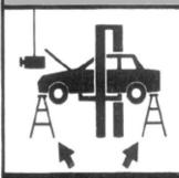
Always use safety stands when removing or installing heavy components. ©
