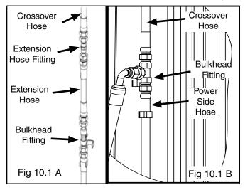
2. Connect the **Power Side** cylinder hose to the tee fitting. Be sure to route the hose through the retainer clips inside the posts.
