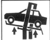
Auxiliary adapters may reduce load capacity.
