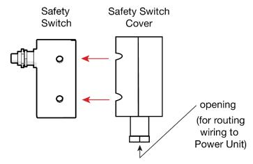
▲ DANGER You *must* attach the Safety Switch Cover to the Safety Switch; without the Safety Switch Cover in place, you could short circuit the electrical components and you could damage the unit or be electrocuted, resulting in serious injury or even death.
