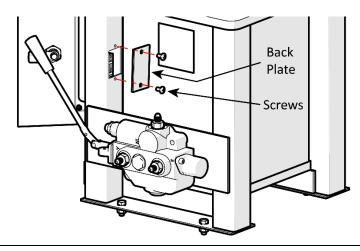
2. Temporarily remove the Safety Switch from behind the door, then attach the wiring cord to the Safety Switch.
