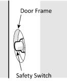
Drawing shows the Switch in place behind Door Frame. Not all components shown.
