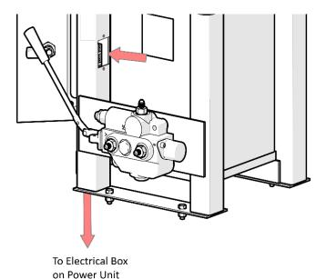
Switch must be **below or flush** with door frame in order for door to close properly
