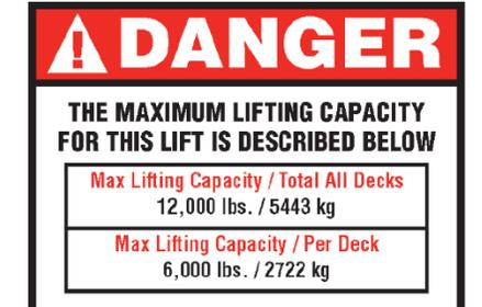
Exceeding the weight capacity of this lift can damage lift and/or property and may cause personal harm, injury or death to operators and/or bystanders. All vehicles MUST be centered on lifting platforms. Damage to lift due to overloading or misuse IS NOT covered under warranty.
