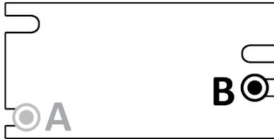
*Drawing shows Button end of Cable B in its slot on the Tie Plate.*
