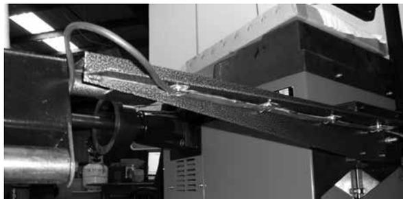
6. Attach the end of the wire to the connection on the back side of the balancer.
