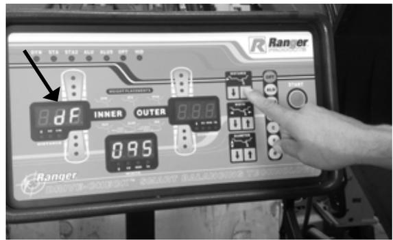
4. Press the **Distance UP Arrow**, four times, until **aut** shows on the inner window. (See below).
