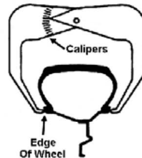
2. Read the measurement for Wheel Width shown on the calipers. (Use the proper scale for Width)
