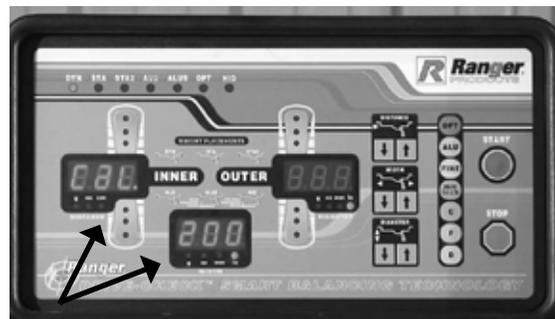
8. Place the tip of the outer gauge arm onto the 200mm calibration attachment mounted on the shaft flange.
