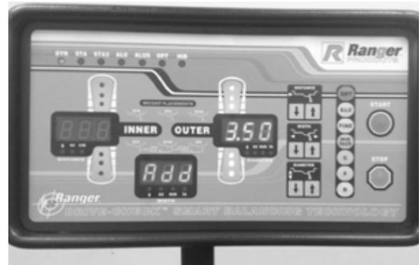
15. Replace weight at the 12 o'clock position on the OUTER side of wheel.
