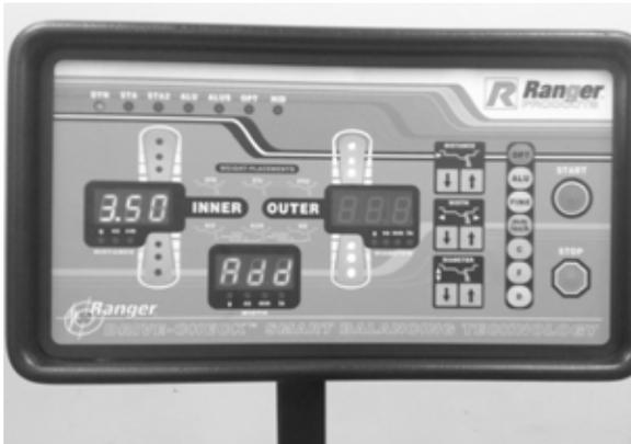
9. Turn the wheel by hand until the weight position indicator lights on the side marked INNER are fully illuminated.
