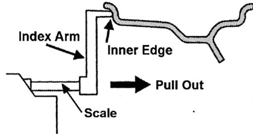
4. Read the offset measurement as displayed on the scale directly on top of index arm. Press the corresponding + - buttons below
