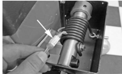
8. Tuck the wire into the Hood Switch Box and install Hood Switch Box Cover and tighten Allen bolts.
