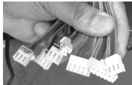
4. Be aware that CN4, CN8, and CN3 located on the bottom right (See image below), are color coded. Plug in these 3 pin connectors to their matching color terminals on the board.
