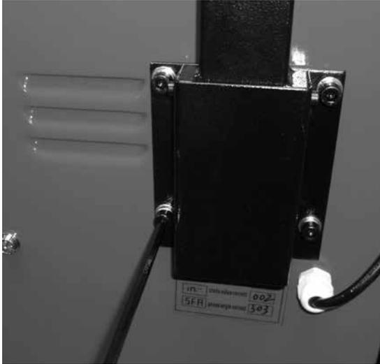
5. Raise the hood and hold it up. Use help to hold the hood while attaching the hood to the Hood Arm.
