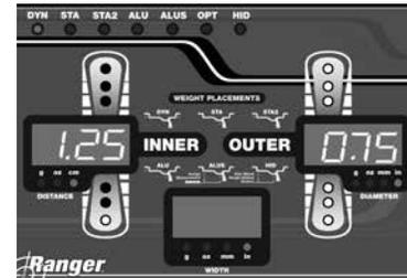
7. Attach the specified weight for the appropriate **PLANE** position at top-dead-center.
