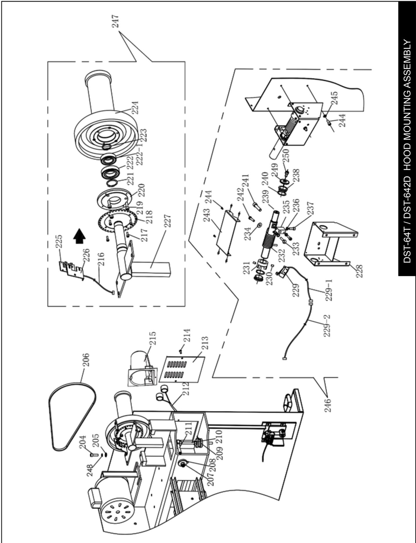
DST-64T / DST-642D HOOD MOUNTING ASSEMBLY
