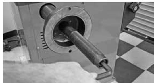
2. Locate and align the mating marks on the Face Plate and Shaft Assembly.
