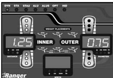
**FULLY ILLUMINATED.** This indicates the position specified by the balancer for the inner weight position.
