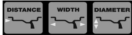
When a wheel is spun, the balancer detects any imbalance present. The computer calculates the weight needed to correct the imbalance and the location for weight application. The weight required to correct the imbalance is displayed on the control panel, and the weight positioning lights assist the operator in positioning the weight application location at top-dead-center. Weight displays and positioning lights are provided for both inner and outer planes of the wheel.
