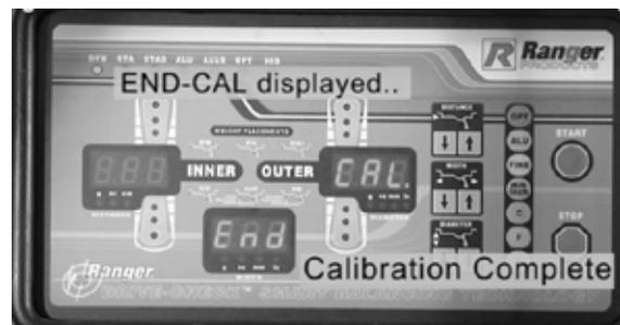
**NOTE:** It is a good idea to keep the known good “calibration standard 18” wheel/tire assembly” set up for the monthly calibration procedure.
