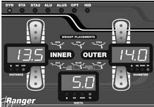
**NOTE:** If this number is not correct you will need to perform the outer gauge arm calibration procedure.
