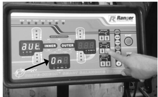
6. Press the **Distance Up Arrow** 3 times to advance to the original start-up balancer screen.
