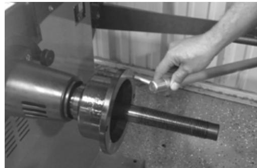
6. While holding the tip of the outer gauge arm onto the shaft flange, press the **ALU** button.
