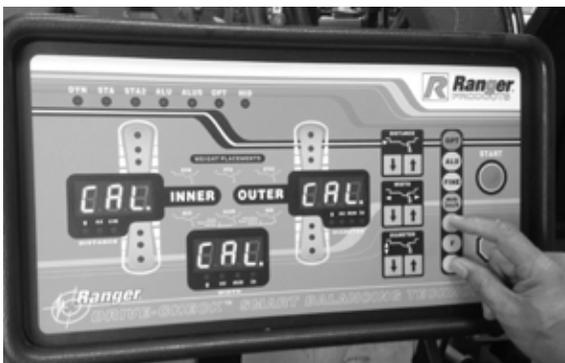
2. Press the **Down Arrow** below distance, then the **Up Arrow** below distance, LED lights will go blank.
