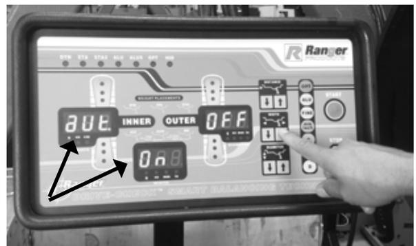
5. If the Width (middle screen) displays OFF, press the Width Arrow UP to change it to ON. If the middle screen displays ON, then the outer arm is already enabled.
