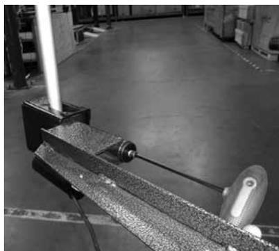
5. Run the wire coming off the gauge-arm through the clips on the underside of the mounting arm.
