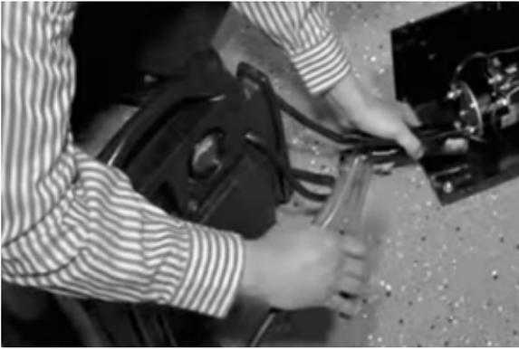
7. Make sure the power unit oil reservoir is full with 2 quarts of automatic transmission fluid
