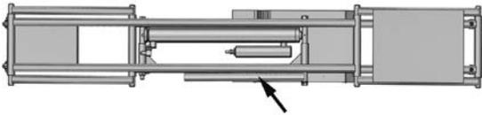
2. Check for proper tension on the safety lock bar retaining nuts. The safety lock bars should remain upright in the stowed position during normal use. They should be manually engaged when required.
