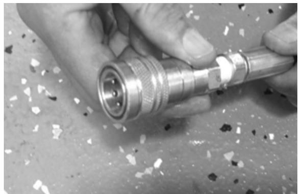
4. Securely tighten female fitting as shown below.
