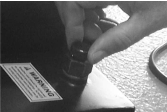
9. Check air pressure in the air bottle cylinders. Make sure both register 50-PSI. **DO NOT EXCEED 50-PSI.**
