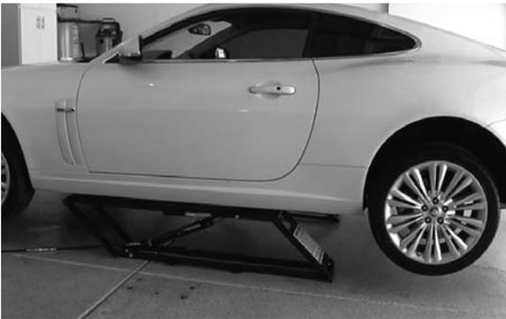
5. Continue to raise to desired height only if vehicle is secure on lift. Keep hair, loose clothing, fingers, and all parts of body away from moving parts. Keep feet clear of jack when lowering. Avoid pinch points.
