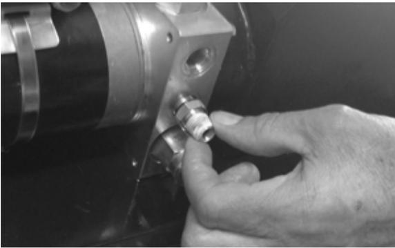
8. Repeat same steps for the upper port. Both fittings should be installed as shown in the images below.
