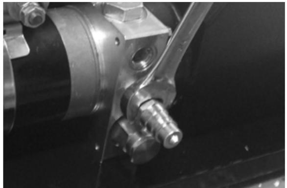
4. Place one double-male O-ring fitting in the lower port, with the O-ring facing inward.
