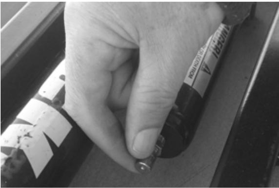
3. If the valve hasn't been opened for a while, use a valve tool to release a short hiss of air to check valve for proper operation and to drain any accumulated oil. Holding the valve open deflates the air bottle cylinder.
