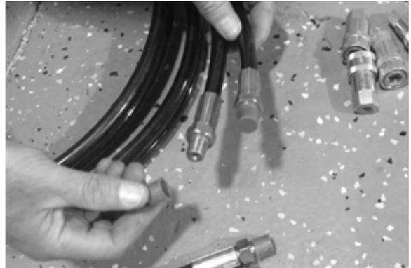
2. Wrap the threads with Teflon tape. When applying tape, wrap it three times in direction shown below.
