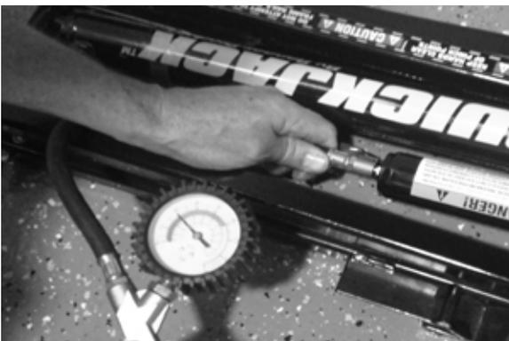
10. Test the Power Unit by pressing the UP button. If the motor sounds like it is operating properly, raise jacks half way and check all hose connections for leaks. If the motor gets hot or sounds irregular, stop and check all electrical connections.
