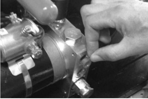
6. Install male quick-connect fitting to lower double-male fitting.
