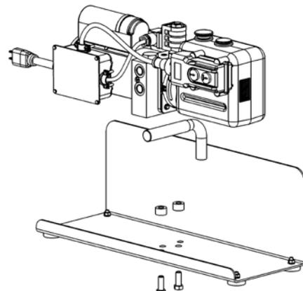
2. Remove protective shipping plugs from both power unit ports.
