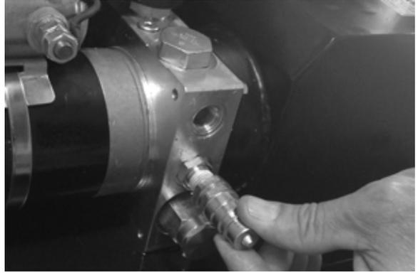
3. Locate both double-male O-ring fittings, then wrap Teflon tape on pipe threads only - NOT O-RING SIDE.
