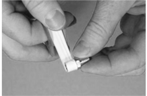
3. Carefully thread each air inflation valve into each air bottle cylinder as shown. NOTE: It is strongly recommended that valve cores be started by hand to minimize cross-threading.
