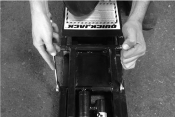
3. Remove any dirt, scales, chips or any foreign debris from your quick-connect fittings to avoid contamination or malfunction of the equipment.
