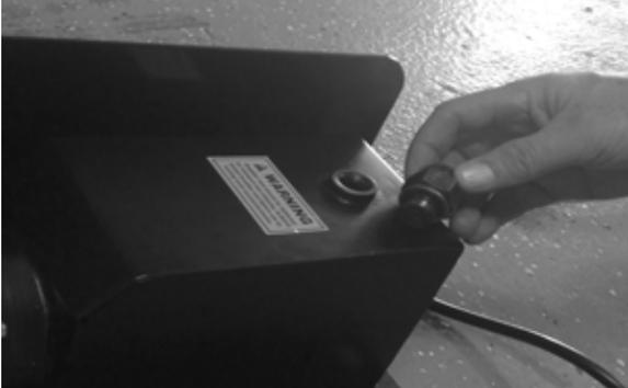
3. Fill the reservoir with approximately 2 quarts of automatic transmission fluid. Make sure the funnel used to fill the power unit oil reservoir is clean.
