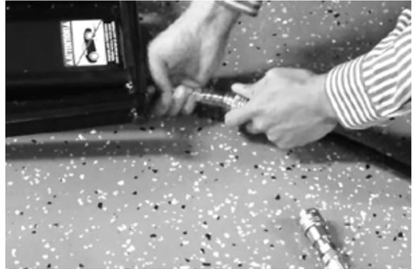
5. For AC Power Units connect directly to a 110-volt power source.
