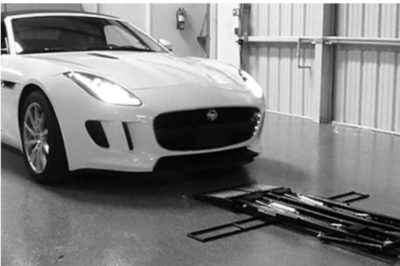
Quick Frame Handles are easily installed by simply lifting the jack frames and placing the end channel underneath the frame tubes as shown below.
