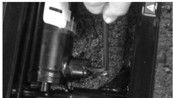
2. Install the 90° O-ring fittings and position the fittings at 10 o'clock.
