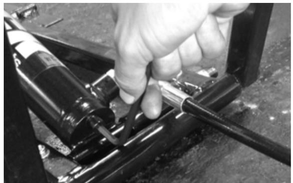
2. Filling: Press the UP button on the power unit pendant control to slowly fill the hydraulic cylinders with oil; air and oil will exit.
