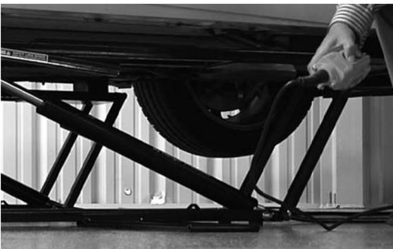
6. Operate the UP control until each jack platform reaches either the low locking position or high locking position.
