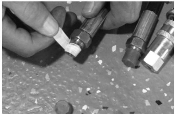
3. Install female quick-connect fitting onto threaded end.
