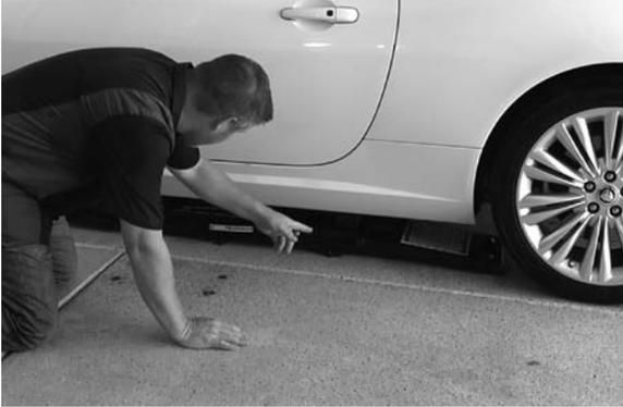
4. When ready, raise vehicle keeping the UP button continuously depressed until tires clear the floor and the jack frames are at least 12" off the ground or the first safety lock position has been reached.
