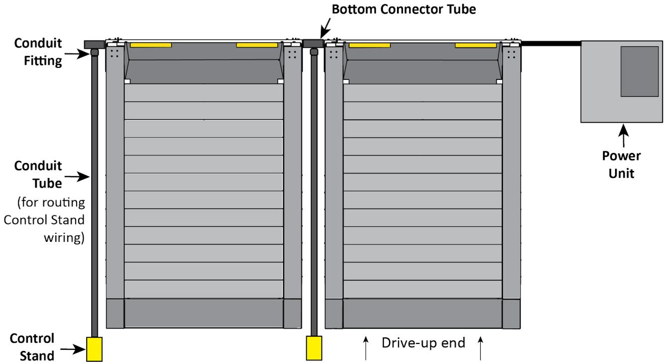
**To install the Control Stand at the *Rear* of the Lift:**
