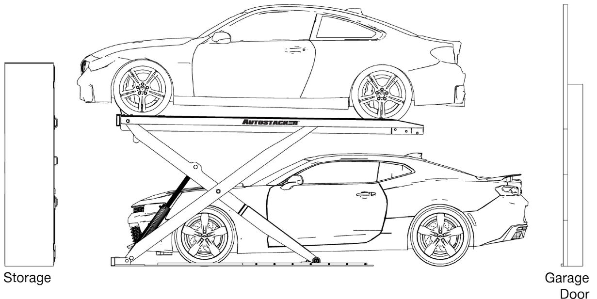
*This image shows an Autostacker using some of the space at the rear (by the garage door) for the Vehicle underneath the Platform to be only partway in.*
