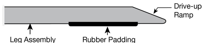
*Not all components shown. Drawing is a side view of the Platform. One Rubber Edge per Leg.*
