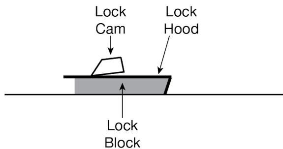
The Lock Hood is securely on the Lock Block.
