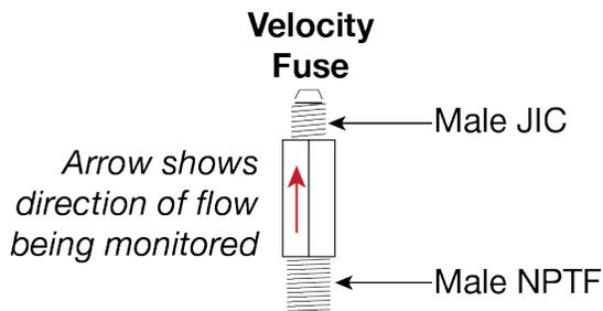
The way a Velocity Fuse works is this: When the Platform is being raised, Hydraulic Fluid moves from the Power Unit to the Hydraulic Cylinder, which uses this force to raise the Platform. When the Platform is being lowered, Hydraulic Fluid moves back from the Hydraulic Cylinder to the Power Unit.
