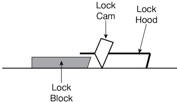
The Lock Hood and Lock Cam move nearly to the next Lock Block in order to disengage completely from the Safety Lock Block it was secured on.
