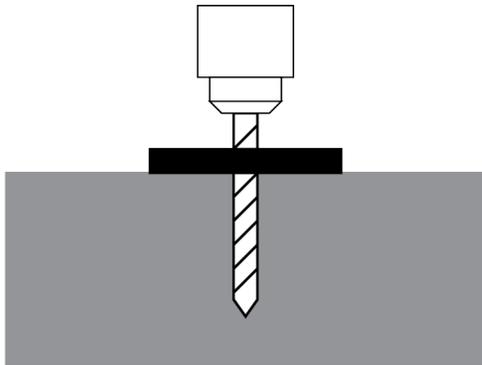
Use a carbide bit (conforming to the current ANSI B212.15).
