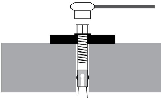
Wrenching the Nut forces the Wedge up, pushing out the Expansion Sleeve and pressing it tightly against the Concrete.
