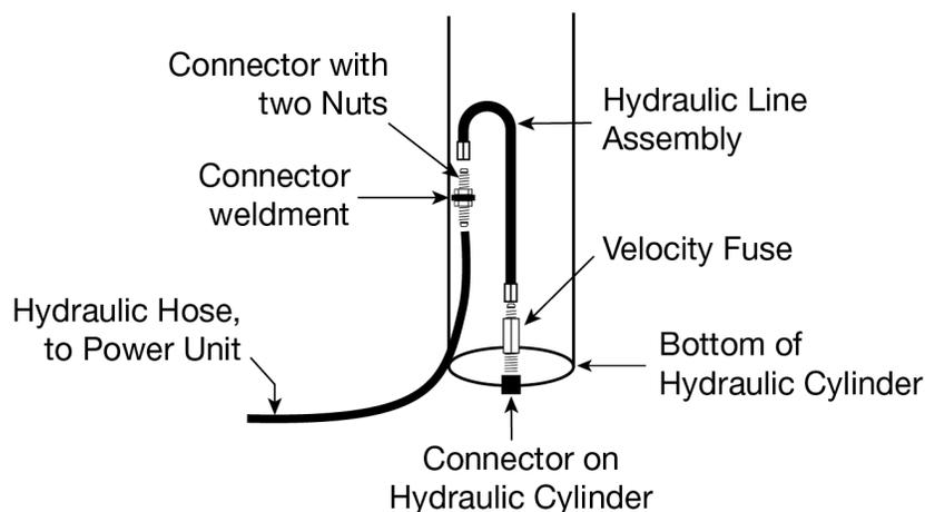
2. On each Cylinder, remove one Nut from the Connector with two Nuts, put the Connector with two Nuts into the Connector Weldment, put the Nut you just removed back onto the Connector with the two Nuts, and finger tighten both Nuts around the Connector Weldment.
