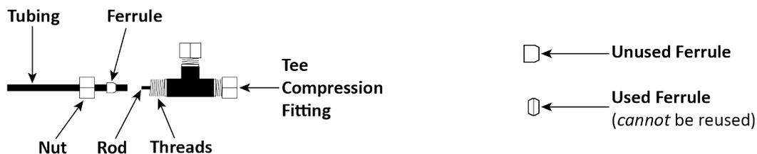
**Important:** *Ferrules can only be tightened once.* When you tighten the Nuts on the Threads, the Ferrules get compressed; it changes shapes and **cannot** be used again.
