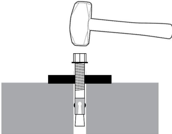
Even using a hammer or mallet, the Anchor Bolt should only go into the Hole part of the way; this is normal. If the Anchor Bolt goes all the way in with little or no resistance, the hole is too wide.
