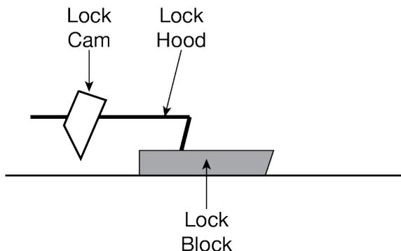
The Lock Hood is partway over the Lock Block; the Lift would **not** go on a Safety Lock at this point.
