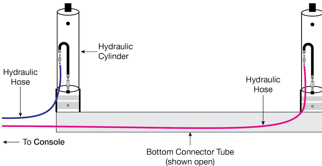
The following drawing is a close-up of the connections to make to the Hydraulic Cylinders.
