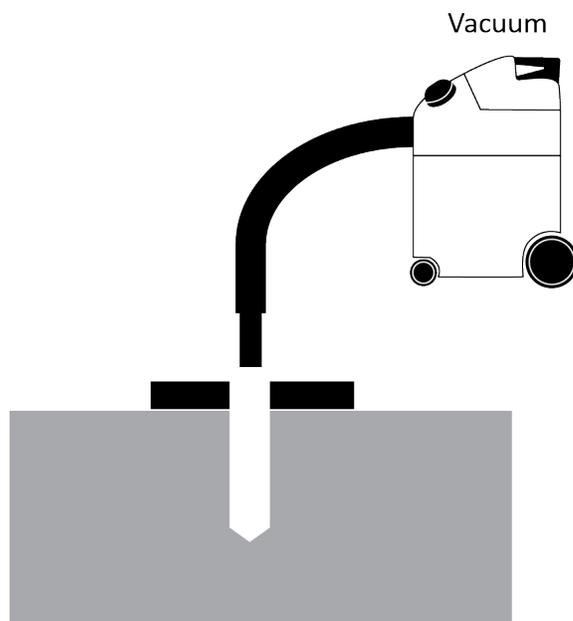
Do **not** ream the hole. Do **not** make the hole any wider than the drill bit made it.
