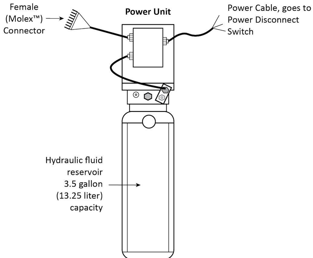
Depending on your Power Unit, the connector locations may be different. Use the drawing below to identify your layout and then attach your Hydraulic Hoses and Return Line appropriately.
