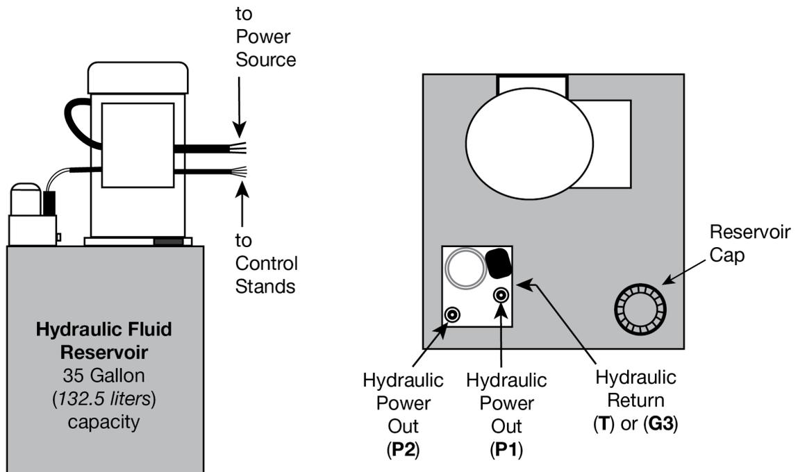
*Drawing not to scale. Not all components shown. Drawing shows top view and side view of the same area. The Hydraulic Return Port is on the side of the Valve Block.*
