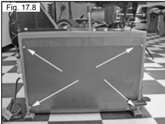
2. Loosen the four Motor mounting / adjusting bolts and nuts. (See Fig. 17.9)
