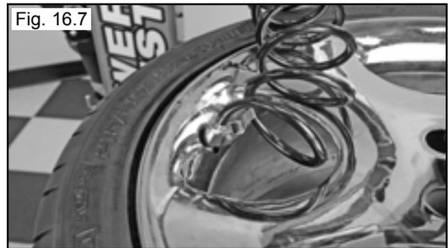
2. Hold tire up against upper edge of the wheel. Be sure tire's top bead is over the bottom of the valve stem. (See Fig. 16.8)
