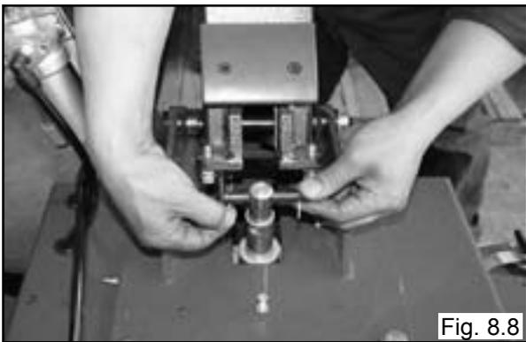
9. Align the Tilt tower and the Safety Hook. Push the Tilt Tower Safety Pin through the Tilt Tower. (See Fig. 8.9)
