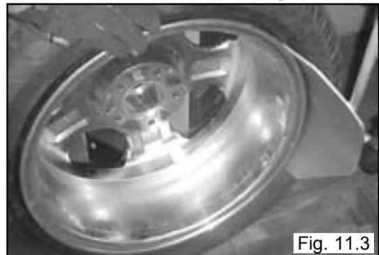
8. Determine the mounting side of the wheel. The mounting side is the narrow side of the drop center. The tire is removed for clarity. (See Fig. 11.4)
