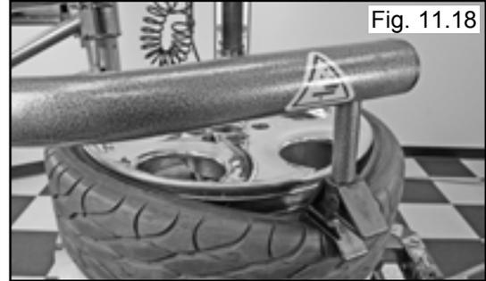
19. Insert the smooth curved end of tool bar over the right end knob of the mount/demount head and below the top bead of the tire. (See Fig. 11.19 -11.20)
