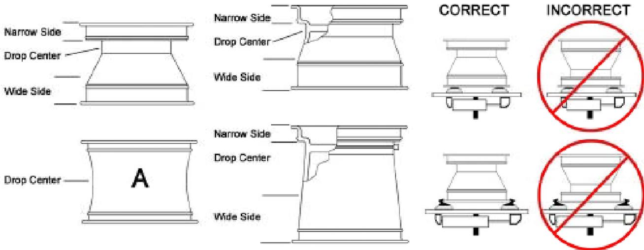
**WARNING!** - The wheel illustrated above in diagram A has little or no prominent drop center. These are not DOT approved wheel configurations. The tire or wheel - or both - can be damaged during mounting procedures causing the tire to explode under pressure, resulting in serious injury or death. If you attempt to mount/demount this type of wheel, use extreme caution.
