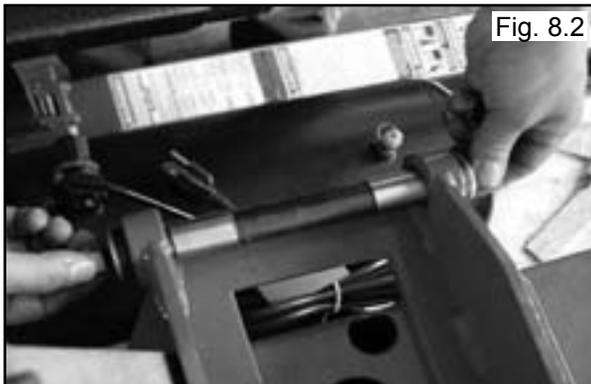
3. Remove the Tilt Tower Safety Pin from the Tilt Tower Base. (See Fig. 8.3)
