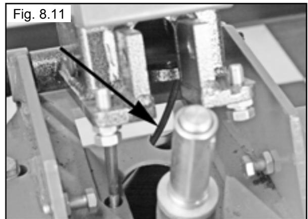
12. Align the Cylinder Shaft and cylinder pin and hole in the Tilt Tower and insert the Cylinder Pin. Secure the Cylinder Pin with the two Cotter Pins and bend Cotter pins. (See Fig 8.12)
