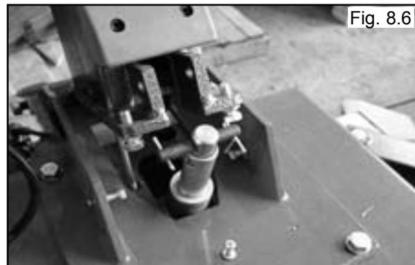
7. Insert the man Pivot Pin through the holes in the Tilt Tower Base and Tilt Tower and secure the Nyloc Nuts. (See Fig. 8.7)
