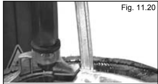
20. Push the tool bar down toward the wheel to lift the tire bead up and over the right -side knob portion of the demount head. Hold the tool bar in this position. (See Fig. 11.21 - 11.22)
