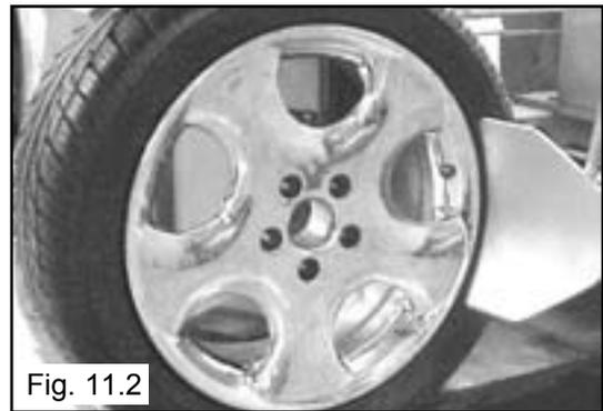
7. Turn wheel around and repeat procedure on the other side of the wheel. This should be the long side of the drop center. It will be easier to clamp the wheel to the table top if the lower bead is loosened last. (See Fig. 11.3)
