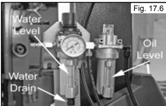
3. Add oil to the lubricator if the fluid level is below the middle of the sight glass. Remove the reservoir by turning counter-clockwise and pulling down. Add SAE 10W non-detergent oil or an air tool oil if necessary.
