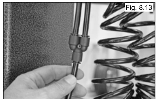
16. Route the Pressure Gauge Air line through the hole in the Base Cabinet and connect it to the Pressure Regulator located at the rear of the Cabinet.
