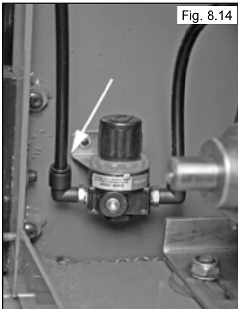
17. Connect the Air Line from the Tilt Back Tower to the Tee Fitting located Inside the Rear of the Cabinet.
