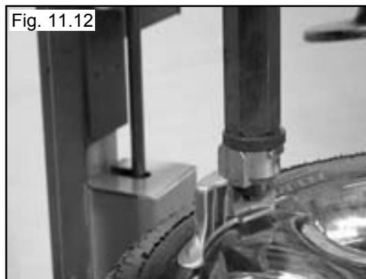
15. Push the locking valve button to lock the slides into place. As the slides are locked, the mount/demount head will move upward approximately 1/8 inch and backward 1/8 inch from the rim edge. The mount/demount head roller should not be in contact with the rim edge. (See Fig. 11.13)
