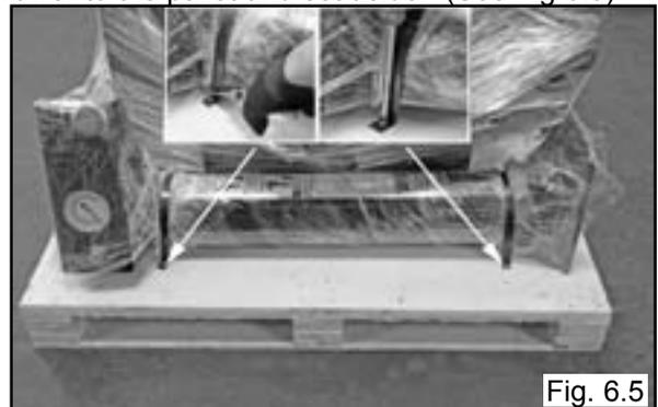
5. While holding the Tilt Tower, carefully cut the Tilt Tower free of the plastic wrapping securing it to the Tire Changer base.
