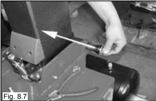
8. Remove the Tilt Tower Cylinder Pin from the Tilt Tower Cylinder Shaft. (See Fig. 8.8)
