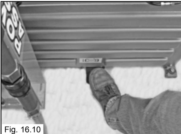
The unit is equipped with a pressure limiter/regulator to assist the operator with proper tire inflation. The pressure limiter will keep most car and light truck tires from inflating beyond 60 PSI (smaller tires may reach higher pressures). It is the operators responsibility to follow all instructions and to control inflation pressure as specified in these instructions. (See Fig. 16.11)
