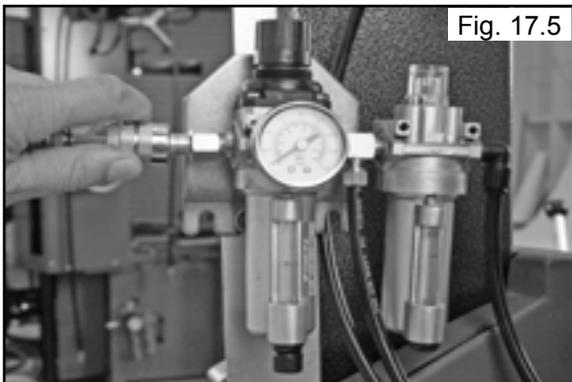
2. Observe the sight glass on the water separator/filter unit. If water is observed, drain by pressing upwards on the drain plug at the bottom of the reservoir. (See Fig. 17.6)
