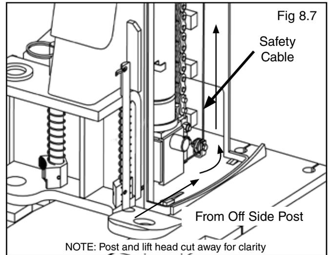
7. Pull the slack out the safety cable and keep tension on the cable as nuts are being tightened. Tighten jam nuts on either side of the cable keeping the cable centered to the hole to secure it into place. (See Fig 8.8)
