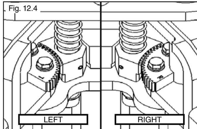
5. Place each Gear Ring against the Lift Head Pin and align the holes in the Gear Ring with the threaded holes in the Arm Ears. Ensure that the teeth on the Gear Ring mesh smoothly with the teeth on the gears of the Lift Head. (See Fig. 12.6)
