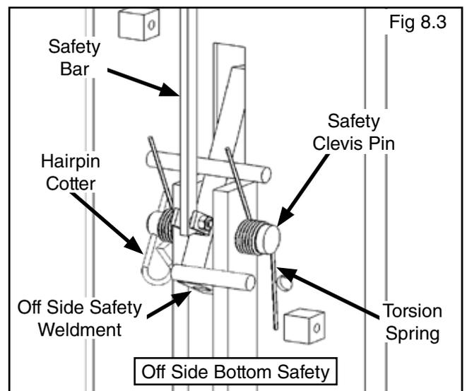
2. From the Off Side post insert the non-looped end of the safety cable through the hole located to the right of the Off Side safety weldment. (See Fig 8.4)
