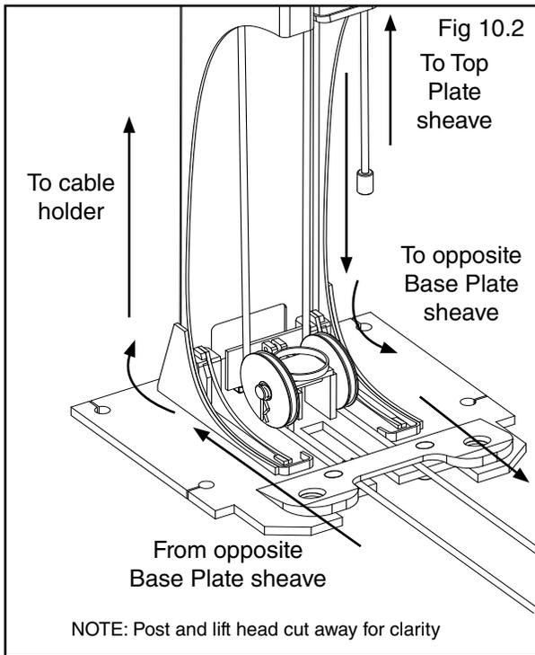
3. Route the threaded cable end to the opposite post's base plate sheave. Wrap the cable around the opposite post's Base Plate sheave and reinstall sheave. (See Fig. 10.2)
