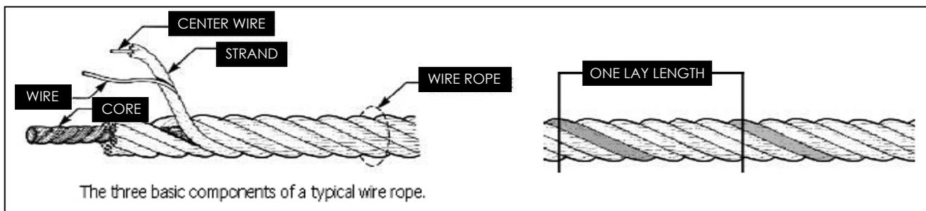
The three basic components of a typical wire rope.
