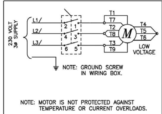
**SEE WIRING INSTRUCTIONS AFFIXED TO MOTOR FOR PROPER WIRING INSTRUCTIONS.**
