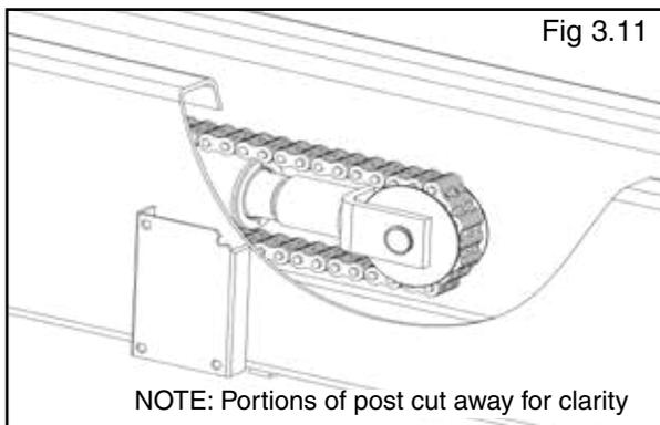
9. Ensure the hydraulic cylinder is properly seated in cylinder ring and that the cylinder leveling plug is installed properly. (See Fig 3.12) Failure to properly align lift head chain and/or cylinder will result in lift malfunction.
