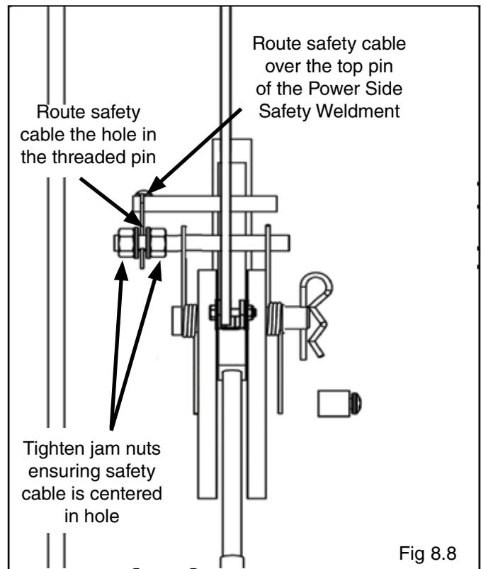
8. Operate the Power Side safety handle, check for proper operation of both safety assemblies and adjust cable tension as required.
