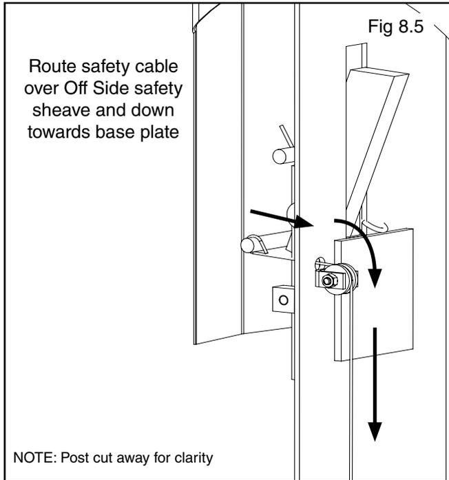
4. Route the cable through the baseplate's safety sheave(s) and across the floor towards the Power Side post. (See Fig 8.6 - 8.7)
