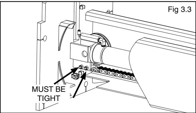
1. With the post assemblies laying on the floor, slide the lift head up towards the top of the post. Inspect and ensure all socket head cap screws and hex nuts are tight. (See Fig 3.1 - 3.3)
