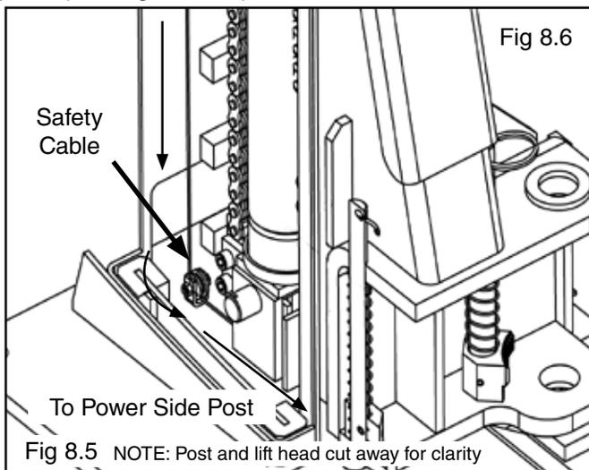
5. Route the cable the same way as on the Off Side going up the post and over the safety cable sheave.
