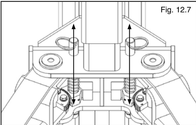
7. Ensure that the arms do not move when a force of approximately 100 pounds or less is applied laterally to the fully extended arms.
