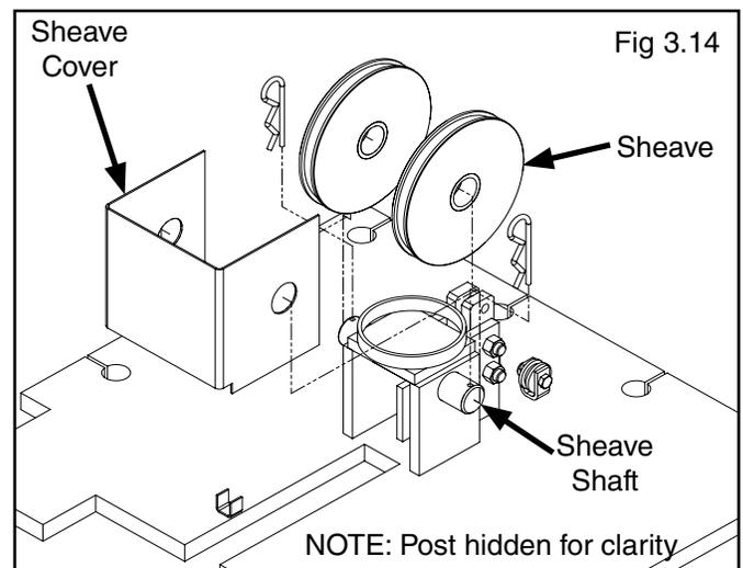
To install optional sheave covers, first fit sheaves over sheave shafts. Then fit sheave cover over both sheave shaft ends. Ensure the notched face of the sheave cover faces the base plate. Secure sheave cover by inserting cotter pins through the cotter pin holes in the sheave shaft.
