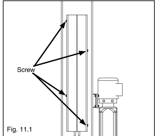
2. Install the floor plate between the columns as shown. For Wide configuration use the floor plate extension. (See Fig. 11.2)
