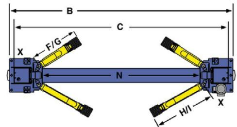
NOTE: Power unit can be located at either X location.
