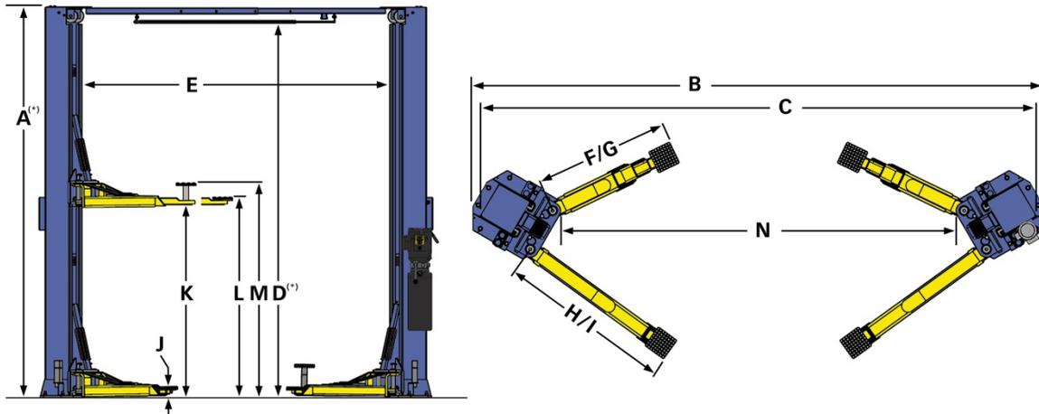
MODELO DOS POSTES / CARGA PESADA / ASIMETRICO
