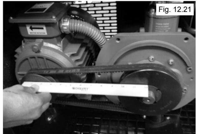
4. Tighten the Mount Bolts and adjust Pulley Tension as described in procedure below.
