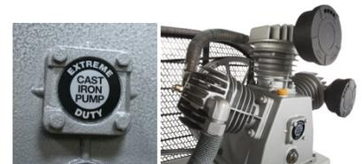
Large "finned" copper tubing helps air stay cool between stages then to tank.
