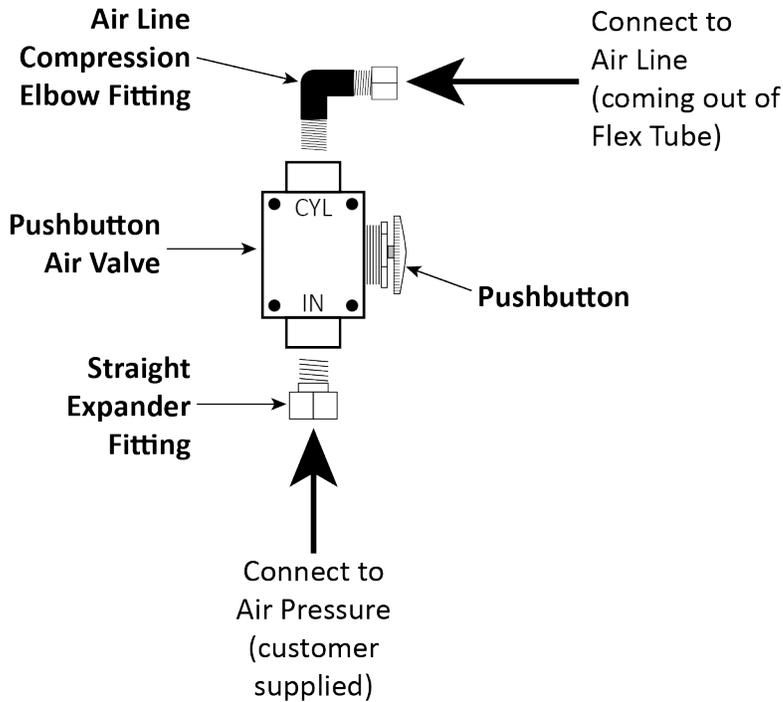
3. Connect the Air Line Compression Elbow Fitting and the Straight Expander Fitting to the appropriate locations on the Pushbutton Air Valve.
