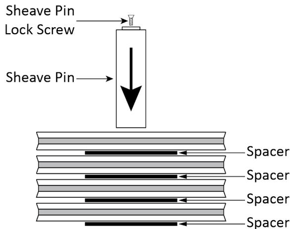
*Drawing shows Sheave Pin being pushed down into the four Cable Sheaves at the Rear of the Lift.*
