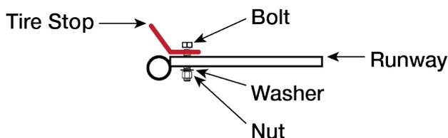
**Note:** Make sure to orient the Tire Stop so that it is sloping away from the Runways. This creates an angle best suited to holding the Tire in place.
