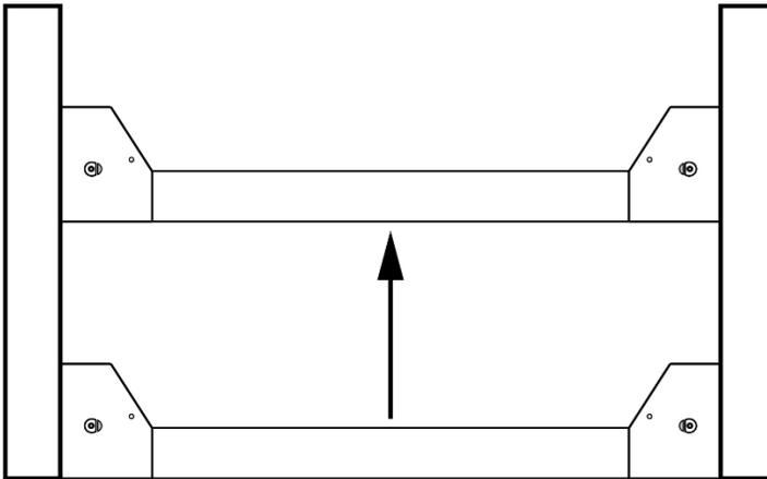
**Important:** Because the Cables are not in place yet, the Slack Safeties are going to engage when you manually raise the Crosstubes. They cannot stay engaged as you continue with the installation; you need to disengage them right after you raise the Crosstubes. The Primary Safeties are not impacted; they will engage normally when you manually raise each Crosstube, which is what you want.
