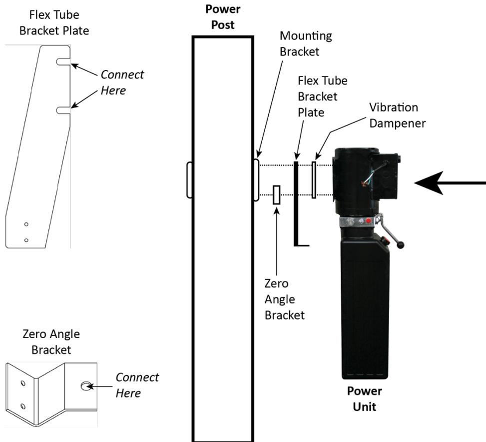
*Drawing combines front and side view. Drawing not to scale. Not all components shown.*
