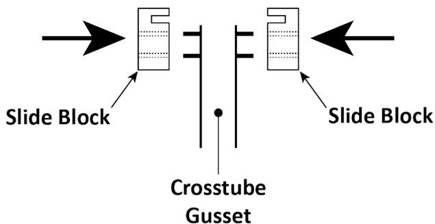
The four Slide Blocks on a Gusset, when put into place, create two Slots. There is one Slot at the top of the Gusset and a second Slot at the bottom; the Ladders, when you install them, **must** go through **both** Slots on the Gusset.
