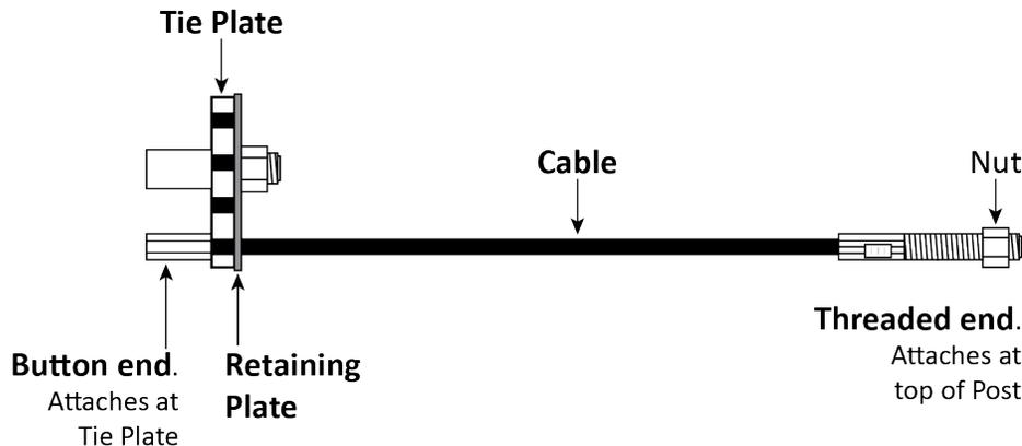
*Drawing not to scale. Not all components shown. The Tie Plate, located under the Powerside Runway, comes attached to the end of the Piston Rod on the Hydraulic Cylinder.*
