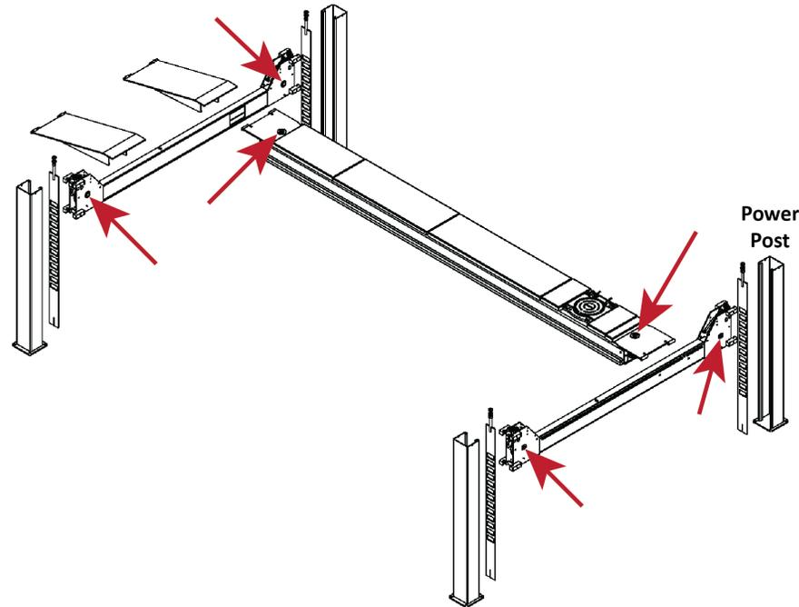
Put a small amount of white lithium grease or similar on each lubrication point before you use the Lift and monthly after putting the Lift into service.
