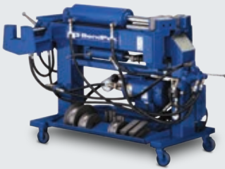
Bending Controls - Manual Clampless Swager - Internal Expander BB-1 Die Package Available
