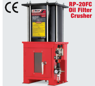
RP-20FC Capacity - 10 Ton / Cycle Time - 15 - 20 sec. Air Requirements - 125 - 175 psi Dimensions - 17" x 29.5" x 17"
