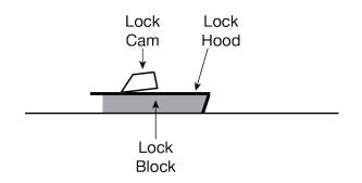
The Lock Hood is securely on the Lock Block.
