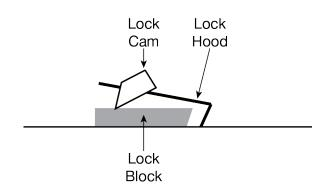
The Lock Hood is at the same level as the Lock Block; if you were to start backing down at this point, the Lift **would** go onto a Safety Lock.
