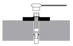
Wrenching the Nut forces the Wedge up, pushing out the Expansion Sleeve and pressing it tightly against the Concrete.
