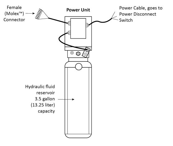
Depending on your Power Unit, the connector locations may be different. Use the drawing below to identify your layout and then attach your Hydraulic Hoses and Return Line appropriately.
