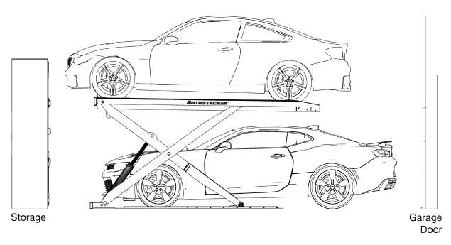
This image shows an Autostacker using some of the space at the rear (by the garage door) for the Vehicle underneath the Platform to be only partway in.
