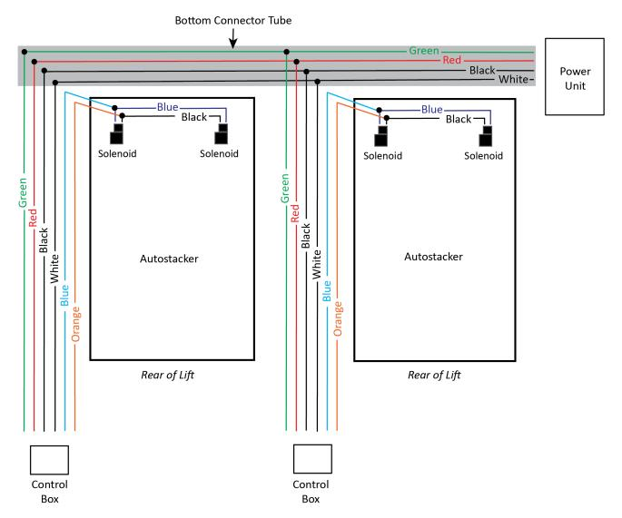
Not drawn to scale. Some components are missing or exaggerated for easier understanding.
