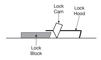
The Lock Hood and Lock Cam move nearly to the next Lock Block in order to disengage completely from the Safety Lock Block it was secured on.
