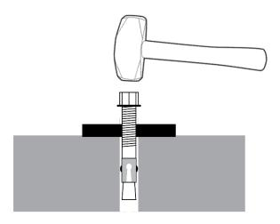
Even using a hammer or mallet, the Anchor Bolt should only go into the Hole part of the way; this is normal. If the Anchor Bolt goes all the way in with little or no resistance, the hole is too wide.
