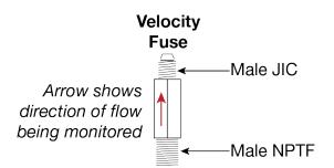
The way a Velocity Fuse works is this: When the Platform is being raised, Hydraulic Fluid moves from the Power Unit to the Hydraulic Cylinder, which uses this force to raise the Platform. When the Platform is being lowered, Hydraulic Fluid moves back from the Hydraulic Cylinder to the Power Unit.
