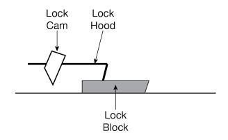
The Lock Hood is partway over the Lock Block; the Lift would *not* go on a Safety Lock at this point.
